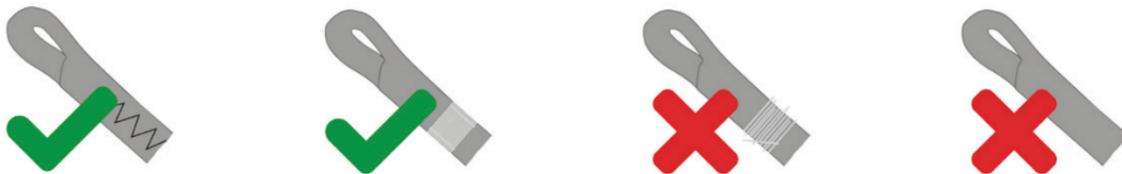
The whipping with lock stitches that prevent the termination from gradually opening must be in place. The eye must not be longer than 25mm (length measured inside the eye). If the cover is damaged, the product must be discarded:
