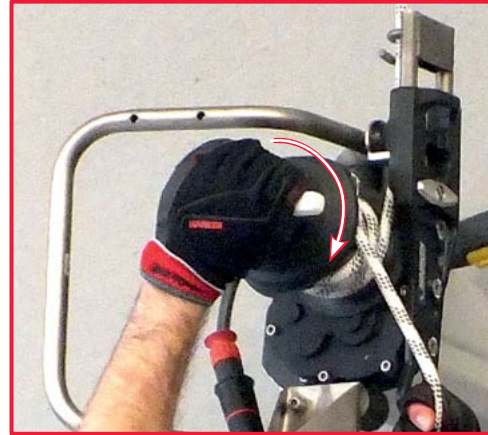
2. With the other hand, turn the control lever clockwise to allow the rope to slip on the winch drum and permit a controlled descent. To adjust descent speed, manually control the speed at which the rope leaves the winch. To stop the descent, release the control lever.
