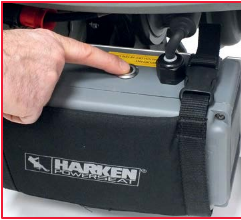
Turn on the battery pushing the power button and check the state of charge.
