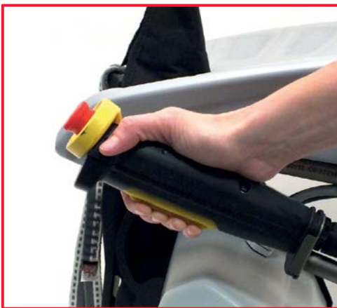
Verify the functionality of the anti-panic system: push the accelerator lever to start the device, and push further the accelerator lever up to the stop, and verify the stop of the device. Release the accelerator lever to disarm the anti-panic system.
