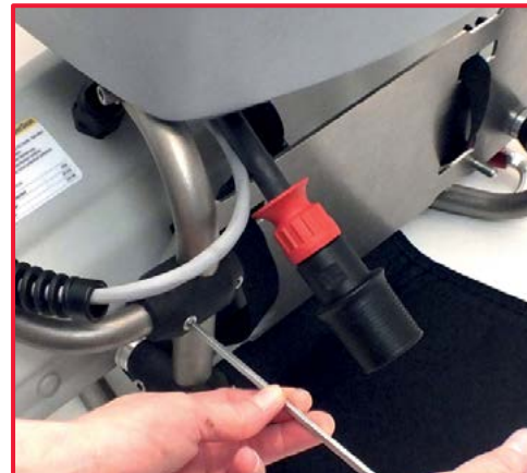
2. Unscrew the second screw in the accelerator control with an Allen wrench no. 4. Please watch out not to lose the self-locking nut.
