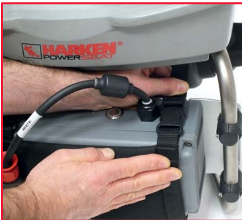
3. Make sure that the hooks of the protective cover is positioned on the flat surface of the battery.
