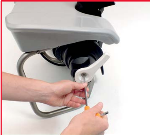
1. Loose the control lever screw using an hex key n°5.
