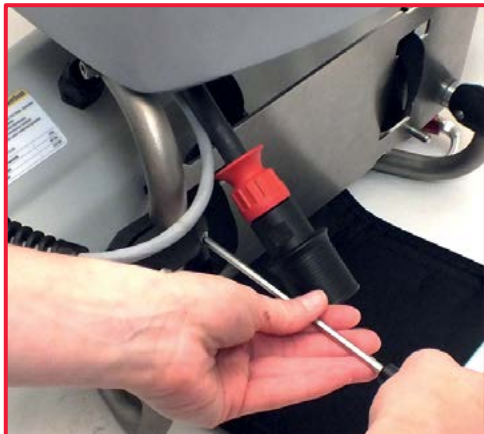
1. After having unplugged and removed the battery, unscrew the (first) anchor screw that connects the accelerator control with the loom.
