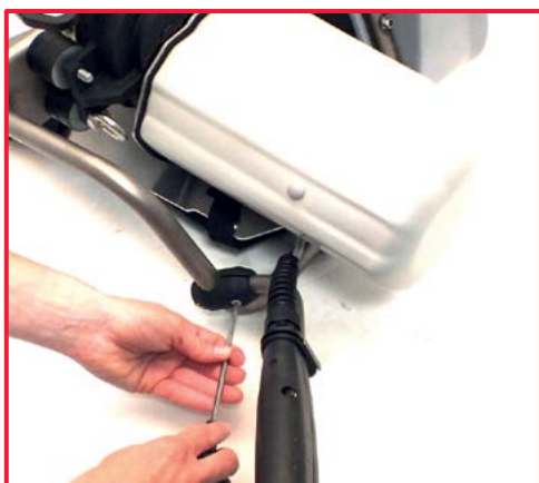
5. Install back the accelerator control in the bearing, and tighten the screws.
