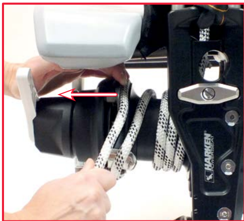
9. Fit the rope into the rope grab. Raise the cover to make this easier.
