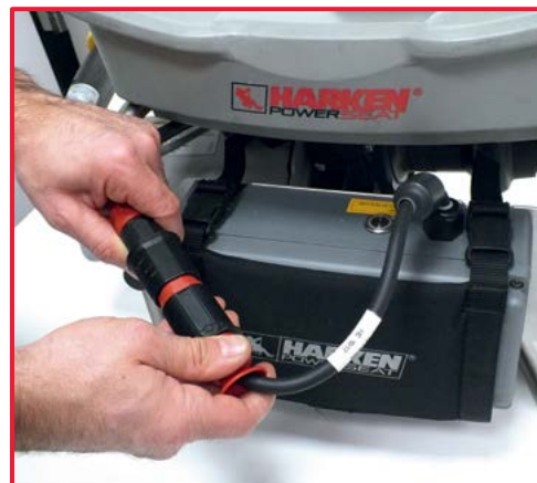
4. Connect the battery grip to the power cable of the motor.
