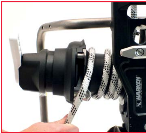
9. Pass the rope over the stripper arm.
