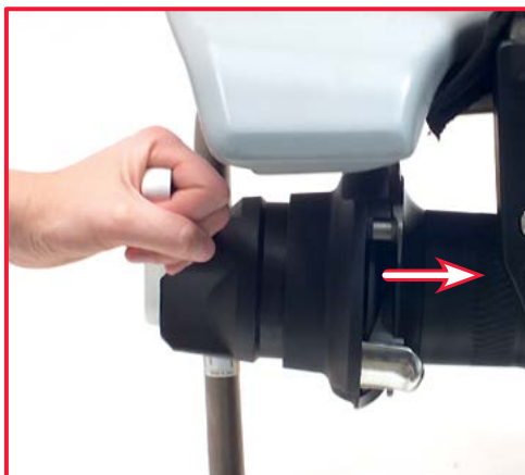
Check that the rope grab knob is working by rotating the control lever and releasing it (CLOSE JAW).
