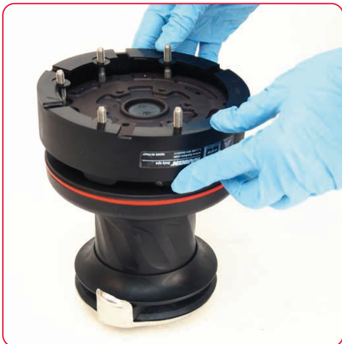
4. Reposition the skirt in its housing
