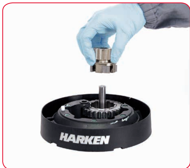
9. Remove the pinion. To facilitate the operation press the spring against the pawl with a blade
