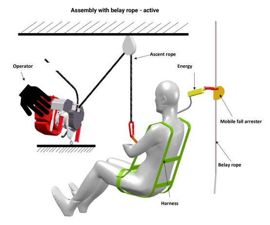
Belay rope type A according to EN 1891 - Observe the operating instructions of the mobile fall arrester and the maximum permissible weight for the energy absorber used.
