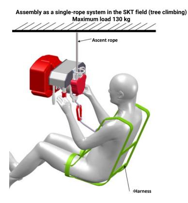
The single rope system is only permitted in the SKT field, i.e. in situations that refer to section 3.4.2 of the German Directive on Industrial Safety and Health (BetrSichV) (e.g. tree climbing). The maximum permissible load for the single-rope system is 130kg.
