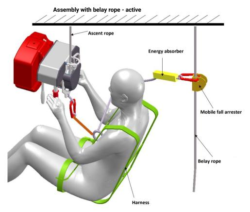
Belay rope type A according to EN 1891 - Observe the operating instructions of the mobile fall arrester and the maximum permissible weight for the energy absorber used.
