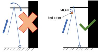
Before each use, check the function of the brake by moving up and down one metre.
