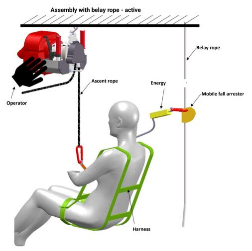
Belay rope type A according to EN 1891 - Observe the operating instructions of the mobile fall arrester and the maximum permissible weight for the energy absorber used.
