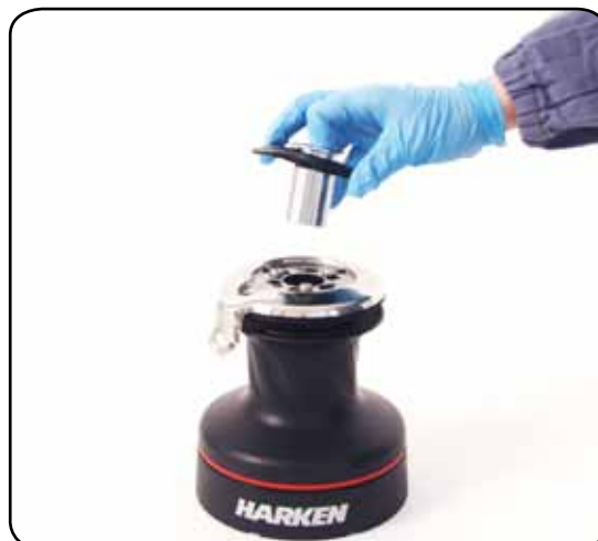
2. Slide off the assy socket n°28 and the cover n°29
