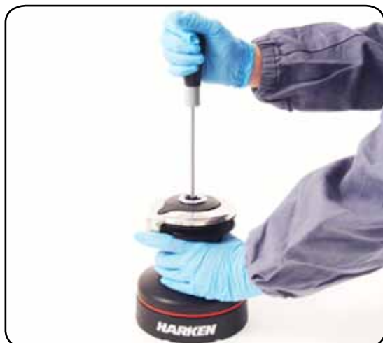
1. Unscrew the central screw ( \approx 2\text{Nm}/18\text{ in-lb} )
