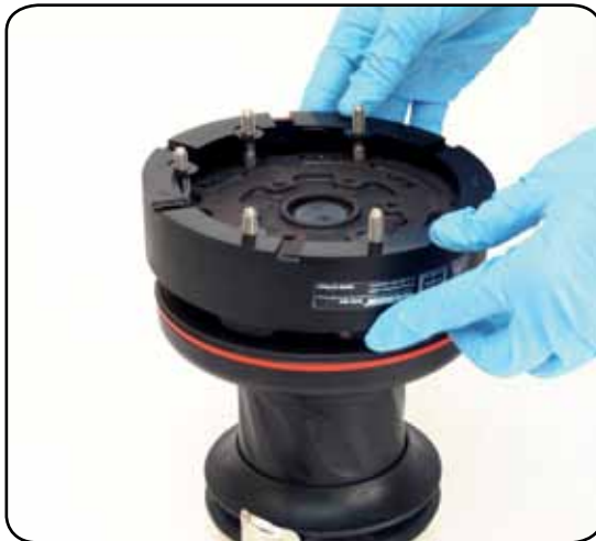
4. Reposition the skirt n°2 in its housing
