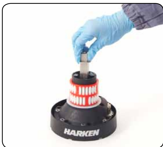
8. Slide out the central shaft n°19
