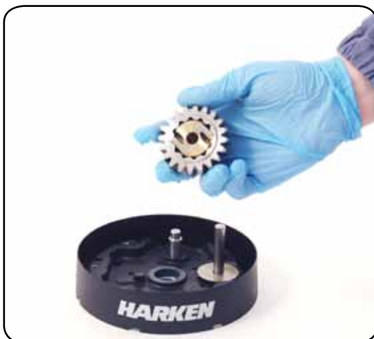
16. Remove the pawls n°5. To facilitate the operation press the spring against the pawl with a blade.
